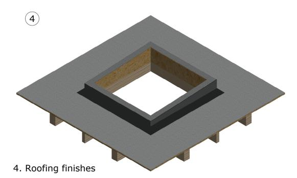
The roofing membrane should not exceed 8mm (including Joints) Should the roofing finishes applied be greater than this then they should be feathered down at the top 50mm to ensure a successfull fitment of the rooflight.
